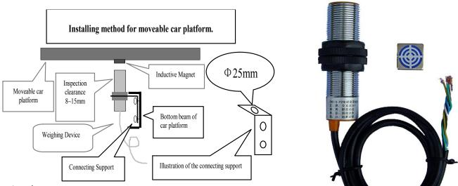
Attention: The system connecting support should be prepared by the customer according to the concrete condition.
